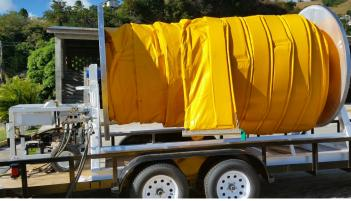
Fast Deployment booms are a must when there is limited storage space, minimal manpower, and or there is a need to deploy the boom as soon as possible.
